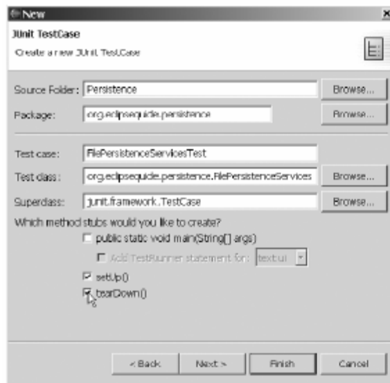
Figure 3.2 Defining the test case and the test class. The JUnit wizard can also provide method stubs for setUp() and tearDown() methods.
